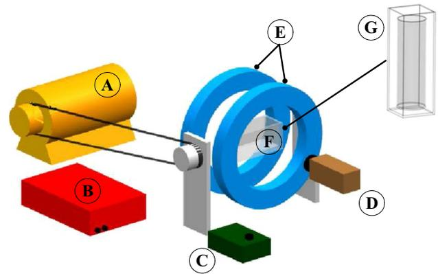
**Fig. 2** Electromagnetic–mechanical device used to actuate the synthetic swimmers. *A* DC motor; *B* DC source to feed coils; *C* angular speed control of the DC motor; *D* digital camera; *E* coil pair; *F* rectangular tank used to test swimmers #1 and #3; *G* cylindrical container used to test swimmer #2 (this cylindrical container was placed in a water-filled rectangular tank to avoid optical aberrations)
